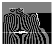
Fig.11. Heat streamlines in a chip mounting
