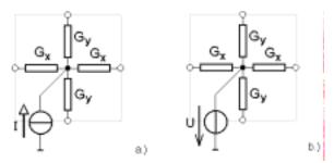
Fig.3. Steady-state circuit models of a single cell.
