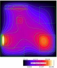
Fig.1. Steady-state temperature distribution on a membrane surface. The rectangular shapes are the dissipating elements.
