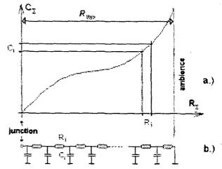
Figure 5 The cumulative structure function of a heat flow path, referring to the partial heat resistances and capacitances, and providing the total  $R_{\rm th}$  of the system
