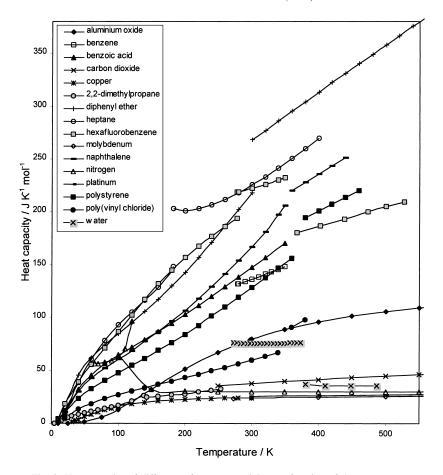
Fig. 2. Heat capacity of different reference materials as a function of the temperature.
