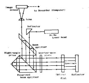
Fig. 2. Optical arrangement of the Type II dilatometer.
