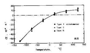
Fig. 6. Linear thermal expansion coefficient α of ULE. The curve —— is merely a guide to the eye.
