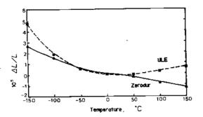
Fig. 5. Linear thermal expansion  $\Delta L/L$  of ULE and Zerodur. The symbols  $\blacksquare$  and  $\triangle$  are these average values from three different dilatometers. The curves —— and —— are merely a guide to the eye.
