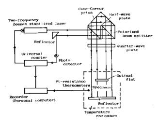
Fig. 3. Schematic diagram of the Type III dilatometer.
