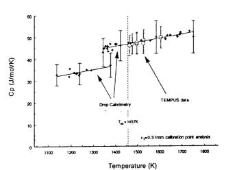
Combined Cp Measurements on Ni<sub>60</sub>Nb<sub>40</sub>
