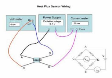
Figure 3. Wire connection with 2 meters
