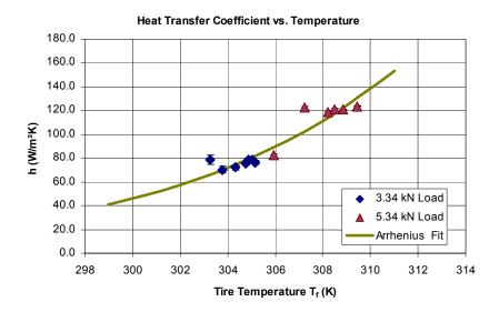
Figure 12: Heat Transfer (Film) Coefficient vs. Tire Temperature T<sub>f</sub>.
