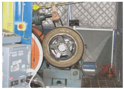
Figure 9. Sensor glued to rolling tire
