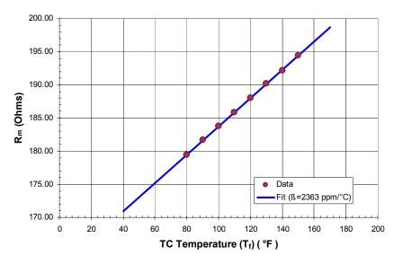
Figure 6. Calibration curve relating bridge resistance to its temperature
