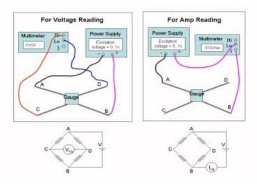
Figure 4. Wire connection with 1 meter
